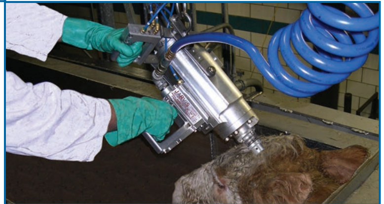
Non-penetrating stunner used with monorail restrainer.
